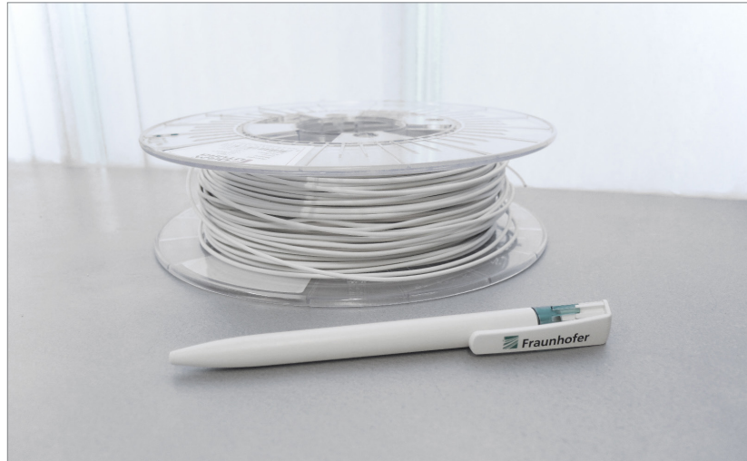
Fig. 8 Filament coil made from INMAFLOW 2010 (Courtesy Fraunhofer IKTS, Germany). This was developed as part of a project supported by Germany's Federal Ministry for Economic Affairs and Energy (BMWi) with the "Zentrales Innovationsprogramm Mittelstand" [1]
