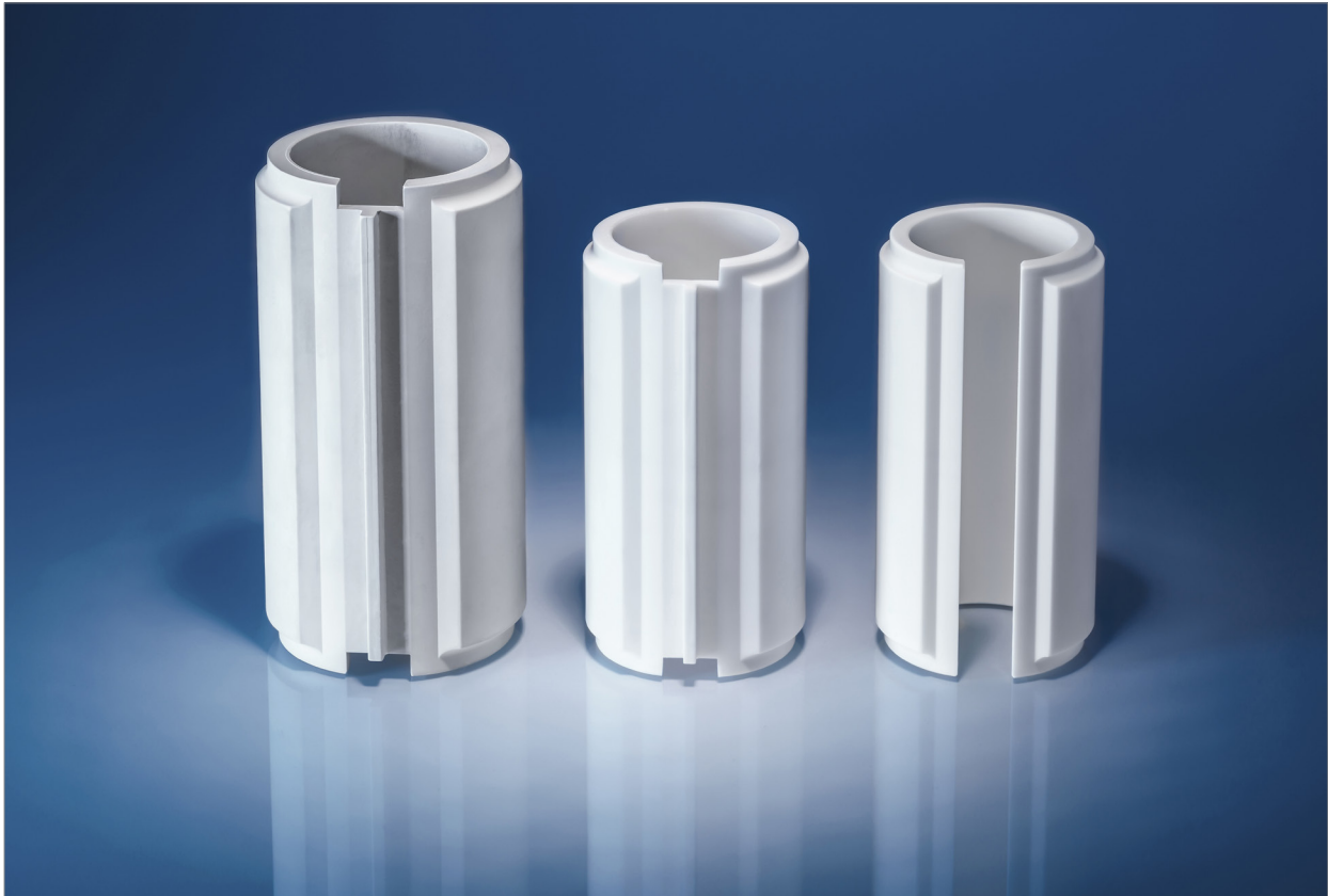
Fig. 2 A CIM thermal insulation tube in the green, sintered and finished states. The tube has been produced with the INMAFEED alumina based feedstock INMAFEED K1008. The dimensions are remarkable: the overall length is 89 mm and the green weight is 335 g (Courtesy Kläger Spritzguss GmbH & Co. KG, Germany)
