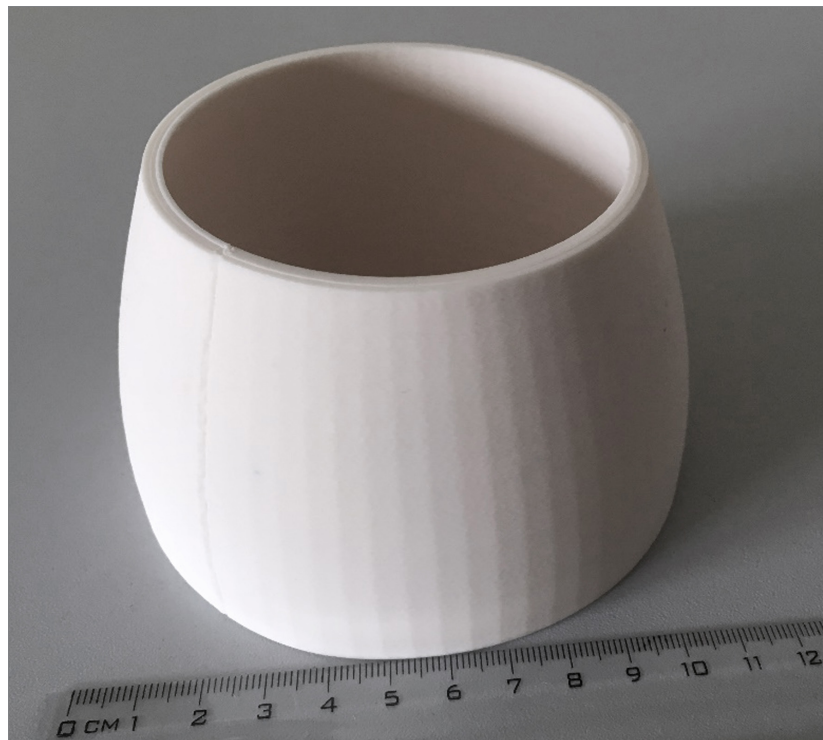
Fig. 9 A sintered Al 2 O 3 laval nozzle made by FFF (Courtesy Fraunhofer IKTS, Germany)
